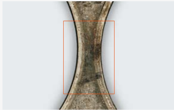
▲ Gas leakage with local blackening of the fire ring bead.
