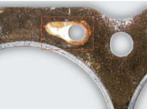
▲ Swelling of composite cylinder-head gaskets due to overheating with steam generation.
