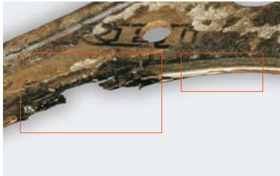
▲ Indentation and crushing due to pre-ignition – with and without blowby.
